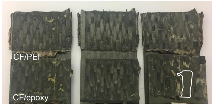
Figure 14: Fracture surfaces obtained from ED-less-250 samples welded at 600 J. Unwelded areas are indicated by the white lines. White arrows indicate locations with discoloured PEI resin.
